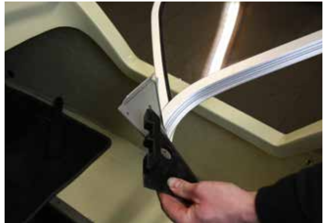
Place the rubber triangles.
