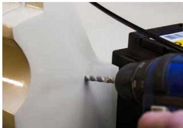
Drill 7.0mm hole for cable.
