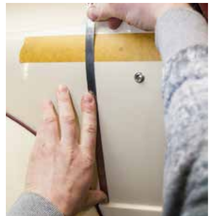
Tape the passenger side and put a line at the edge of the body (241mm).
