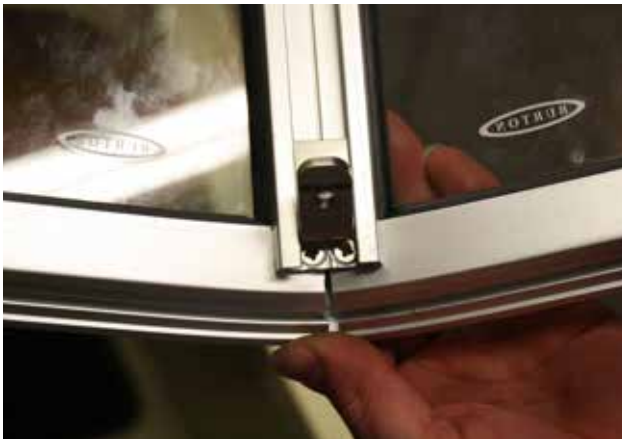
Mount the mounting bracket.
